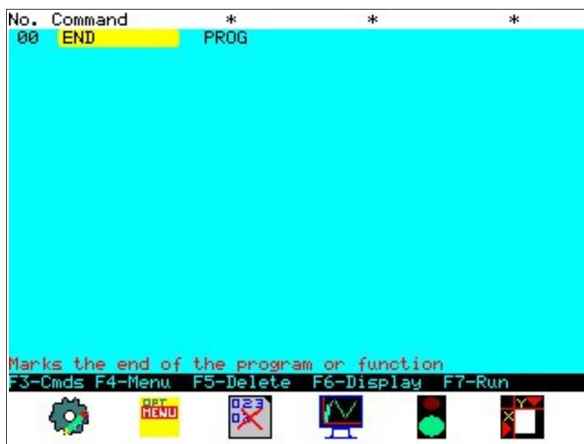
The text in the box at the top of the screen is intended to help with data entry as each command has it's own header. 'No.' represents the line number of the program, 'Command' is the name of the MAP command used and \*,\*,\* are the three heading that will change based on the command. Where a valid command is selected and a column displays '\*', no data should or can be entered.
